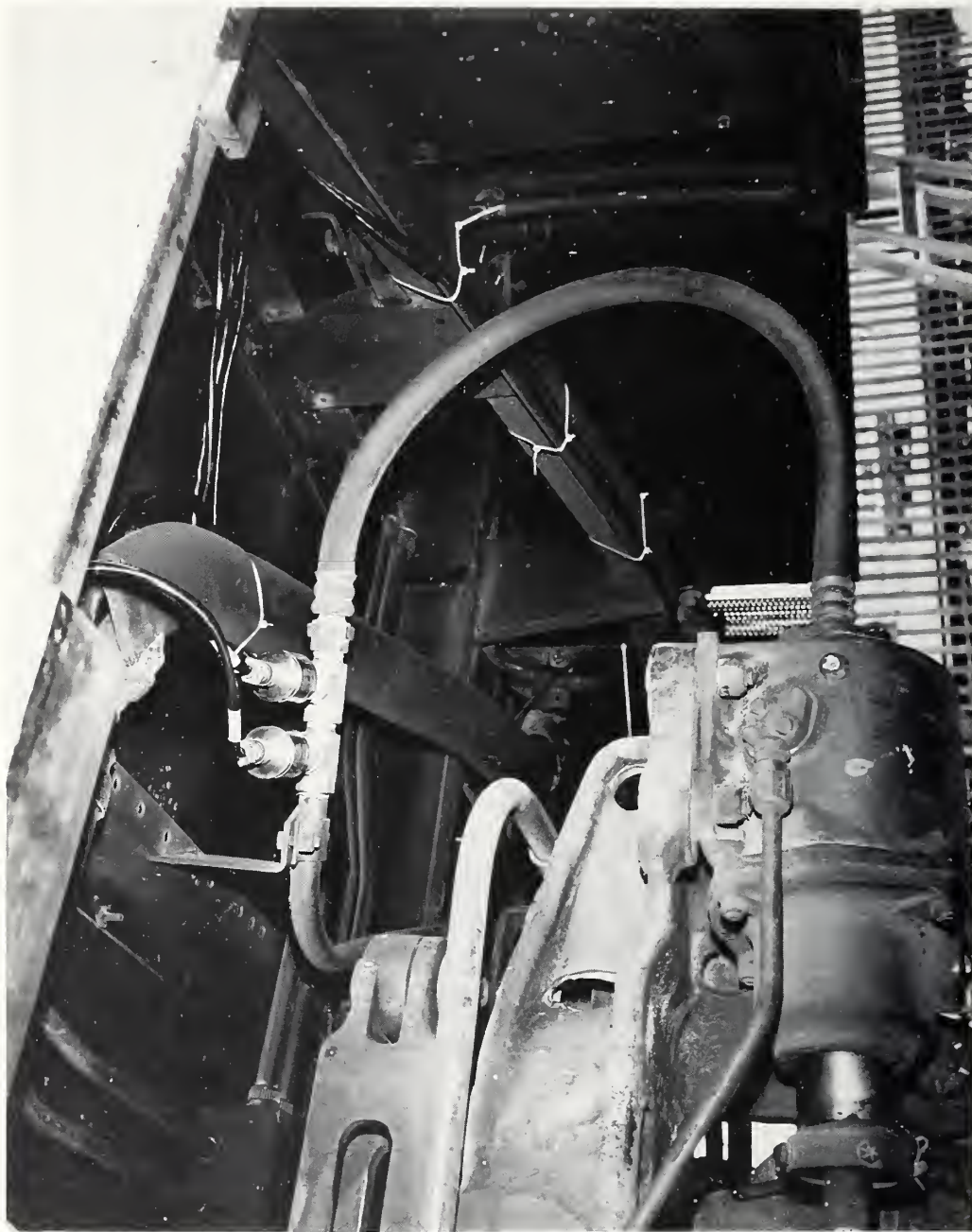
FIGURE D-2. BRAKE PRESSURE SENSOR TEST INSTALLATION, NO. 1 TRUCK
