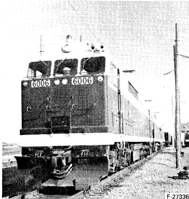
Figure 2-27. General Electric E60C Locomotive in Service at Black Mesa and Lake Powell
