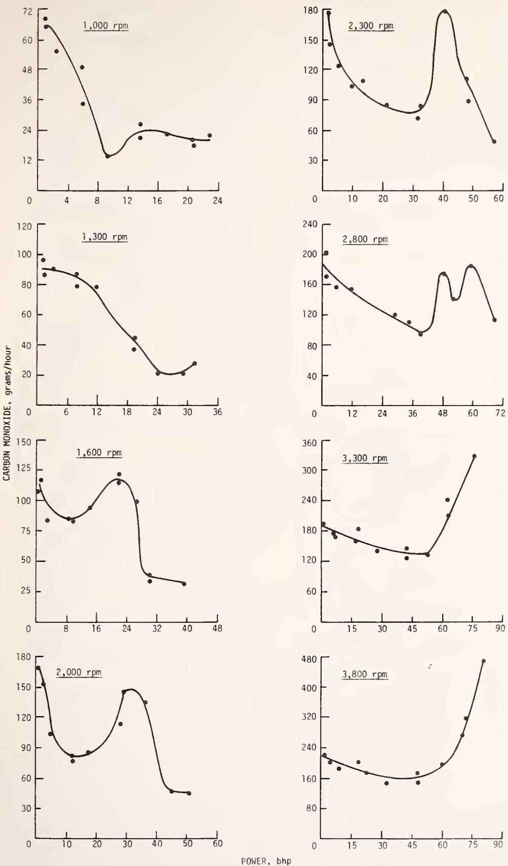
FIGURE 3. Carbon Monoxide Emissions Versus Power at Various Speed and Load Conditions--Chrysler-Nissan Diesel Engine.
