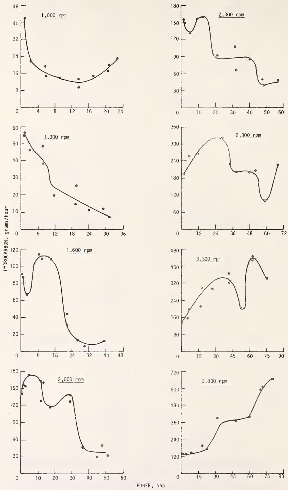
FIGURE 4. Hydrocarbon Emissions Versus Power at Various Speed and Load Conditions--Chrysler-Nissan Diesel Engine.
