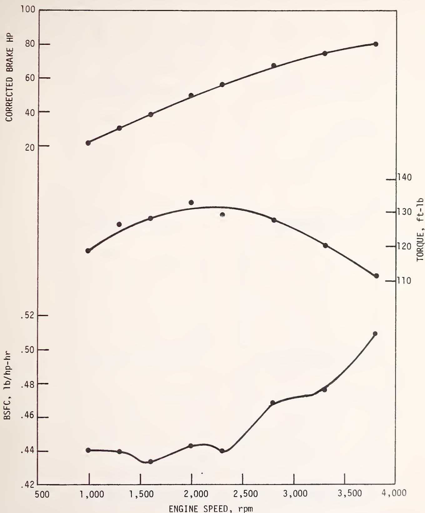
FIGURE 1. Brake Specific Fuel Consumption, Torque, and Brake Horsepower Versus Engine rpm at Wide-Open-Throttle--Chrysler-Nissan Diesel Engine.
