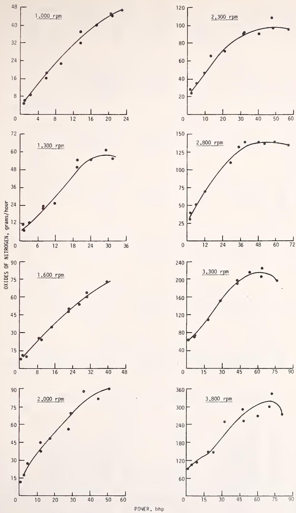
FIGURE 5. Oxides of Nitrogen Emissions Versus Power
