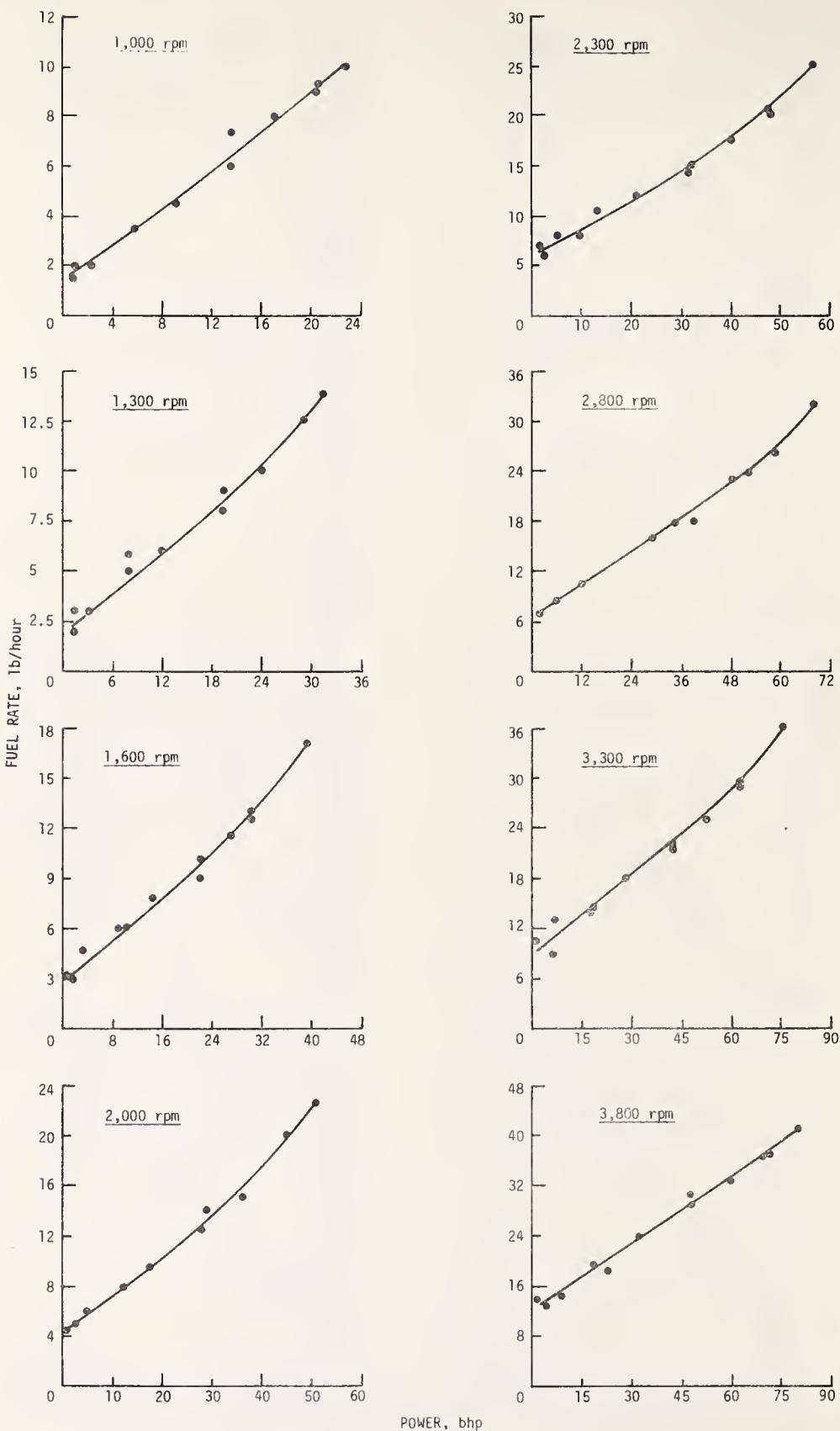
FIGURE 6. Fuel Rate Versus Power at Various Speed and Load Conditions--Chrysler-Nissan Diesel Engine.
