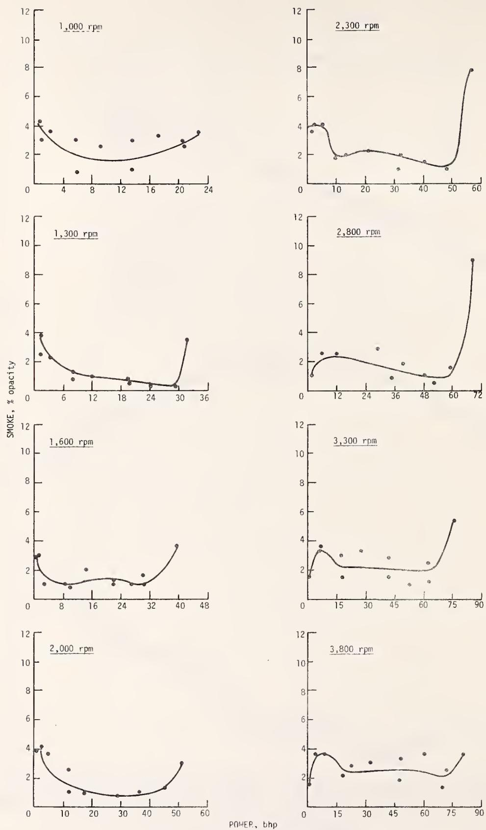
FIGURE 2. Emissions of Smoke Versus Power at Various Speed and Load Conditions--Chrysler-Nissan Diesel Engine.
