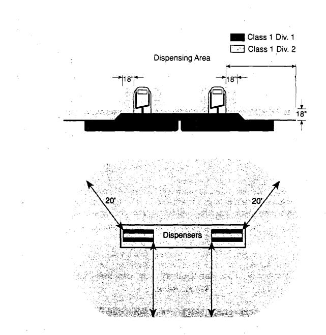
Figure 2-1 Classified Areas Adjacent to Dispensers (Flammable & Combustible Fluids)
