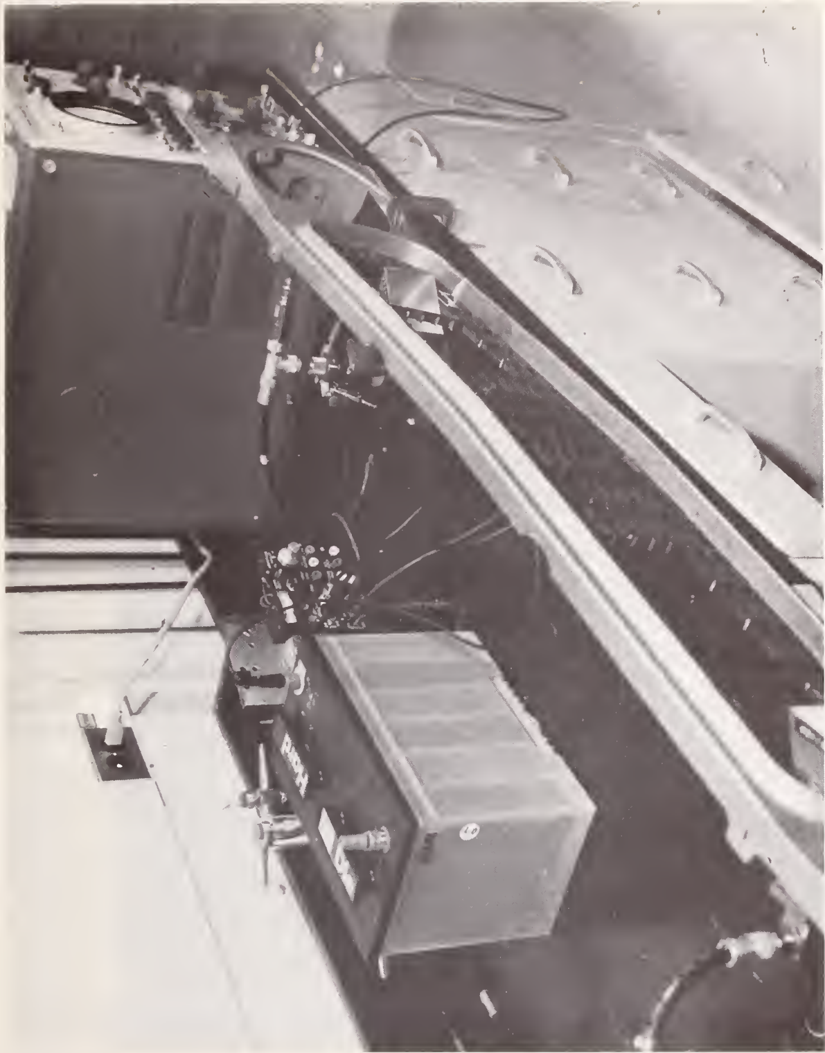
Figure 3-30 Prototype Radar Crash Sensor - Laboratory Model (10 GHz)
