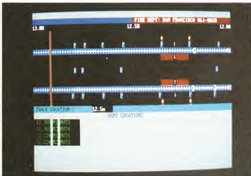
FIGURE 4-11. TRACK DISPLAY: VENT LOCATIONS
