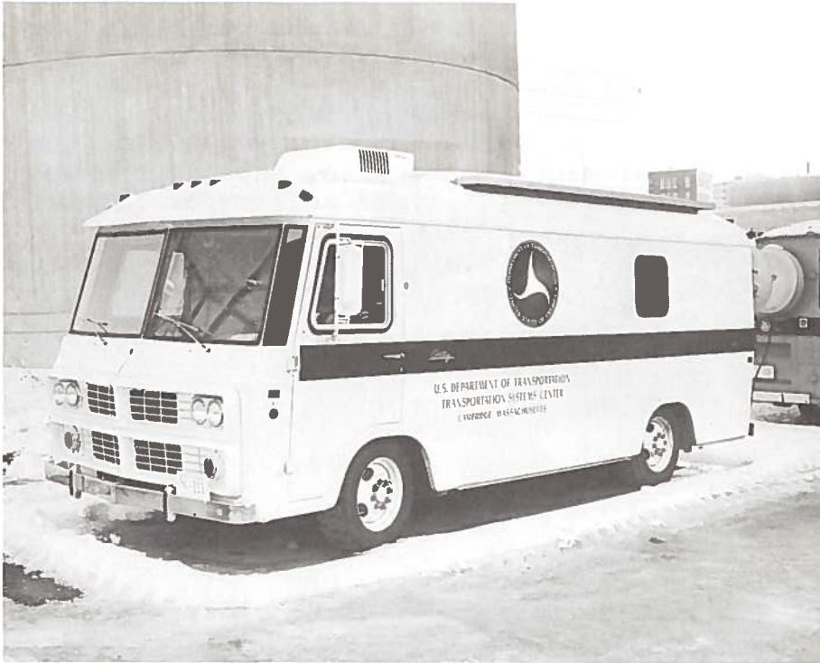
Figure 1-2. Mobile Noise Measuring Van
