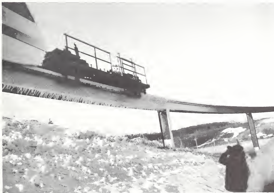
FIGURE 16. RUNNING OVER A GUIDEWAY SECTION WITH SIMULATED BLIZZARD RESULTS
