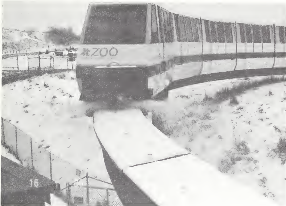
FIGURE 6. PLOW BLADE ELEVATED FOR BRUSH (ONLY) SNOW REMOVAL
