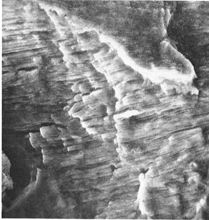
Figure 36.—SEM Micrograph of Steel A Tested in Vacuum. Intermediate - High Growth Rate \Delta K \sim 25 \text{ MN m}^{-3/2}
