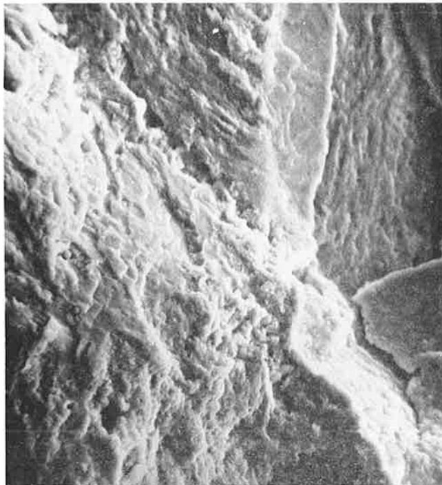
Figure 45.—SEM Micrograph of Steel B Tested in Vacuum. Initiation Region \Delta K \sim 25 \text{ MN m}^{-3/2}
