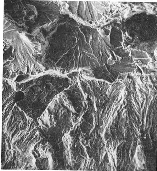
Figure 46.—SEM Micrograph of Steel B Tested in Vacuum. Threshold Region \Delta K \sim 6.5 \text{ MN m}^{-3/2}
