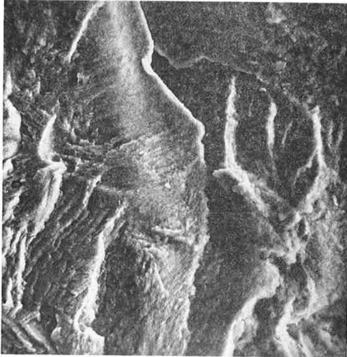
Figure 34.—SEM Micrograph of Steel A Tested in Vacuum. Threshold Region \Delta K \sim 9.5 \text{ MN m}^{-3/2}
