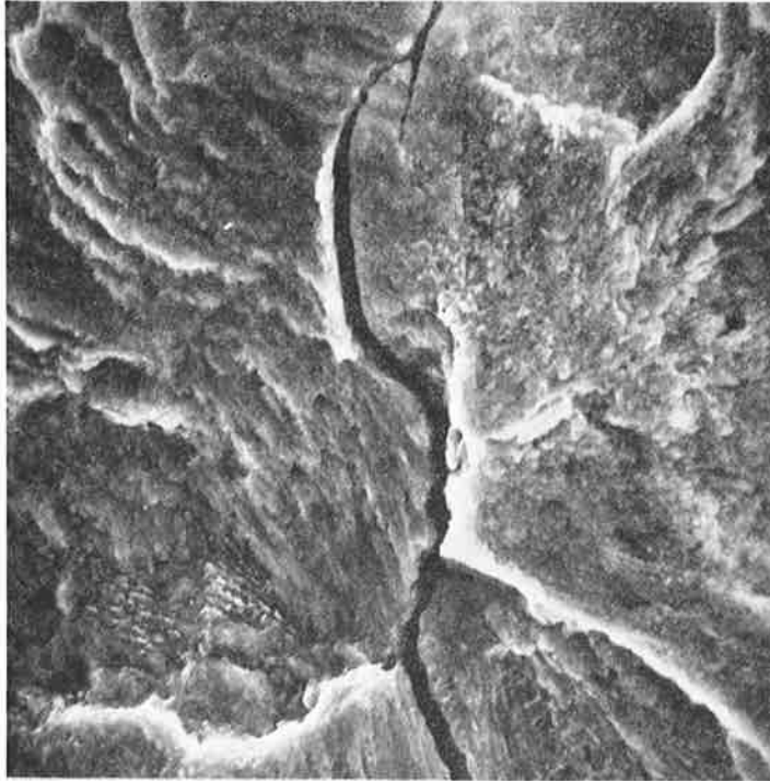
Figure 38.—SEM Micrograph of Steel A Tested in Vacuum. Intermediate Growth rate \Delta K \sim 13 \text{ MN m}^{-3/2}
