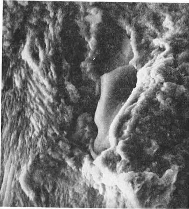
Figure 46.—SEM Micrograph of Steel B Tested in Vacuum. Threshold Region \Delta K \sim 6.5 \text{ MN m}^{-3/2}
