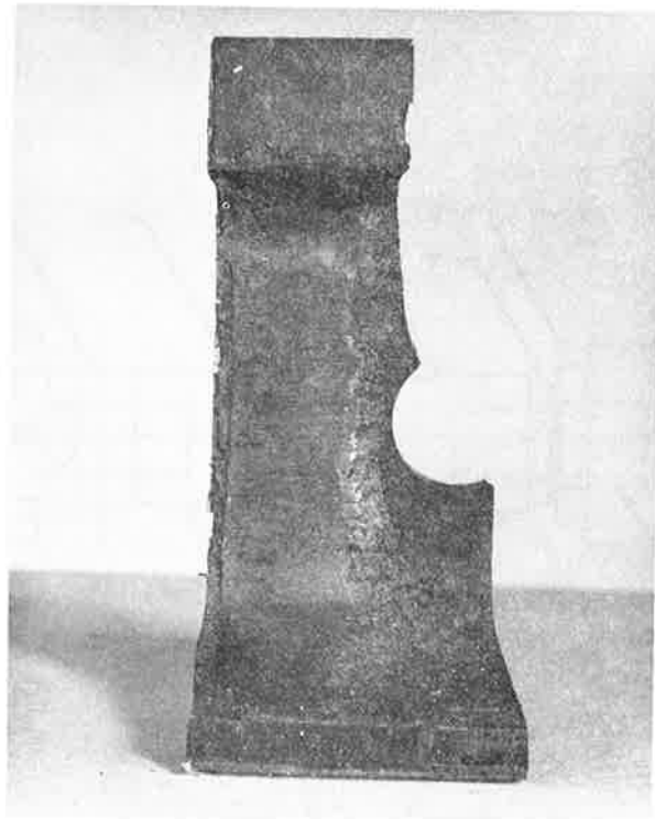
Figure 5.—Sleeve-Expanded Bolt-Hole/Weld Relationship
