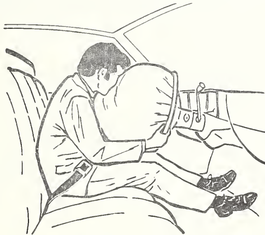
DRIVER SIDE (Air bag in Steering Wheel— Steering Column Absorbs Energy)
