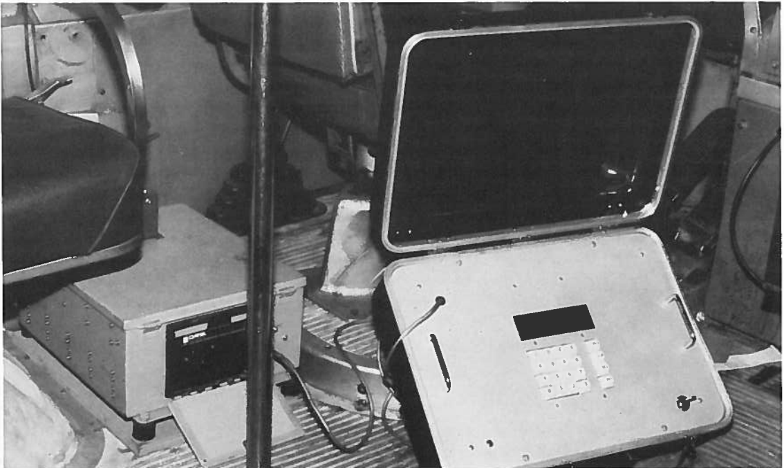
The portable data collection unit demonstrated in Columbus provides information on passenger loads, run times, and schedule adherence. (Photo by General Motors)
