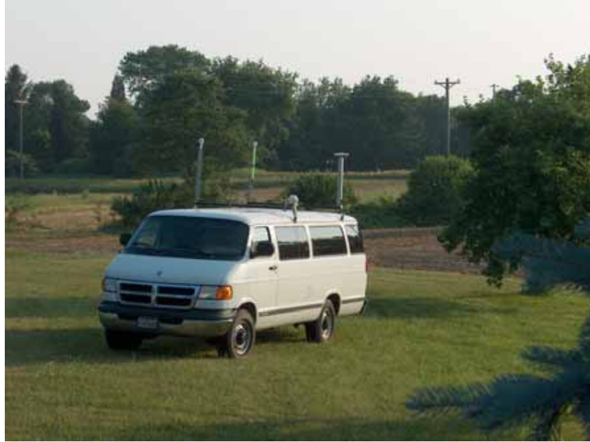
Figure 8. Antenna configuration on van used for collecting data broadcast from HAG1 and HRN2 simultaneously. The van is equipped with one GPS marine antenna and two demodulator receiver antennas.
