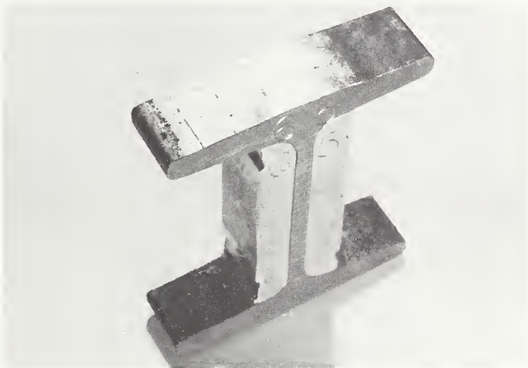
FIGURE 20 THIRD RAIL HEAD AFTER TWO MILLION SHOE PASSES
