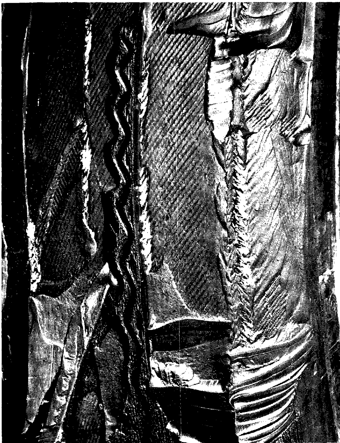
Figure 6. Burnt Mold Groove Line T5X 1223
