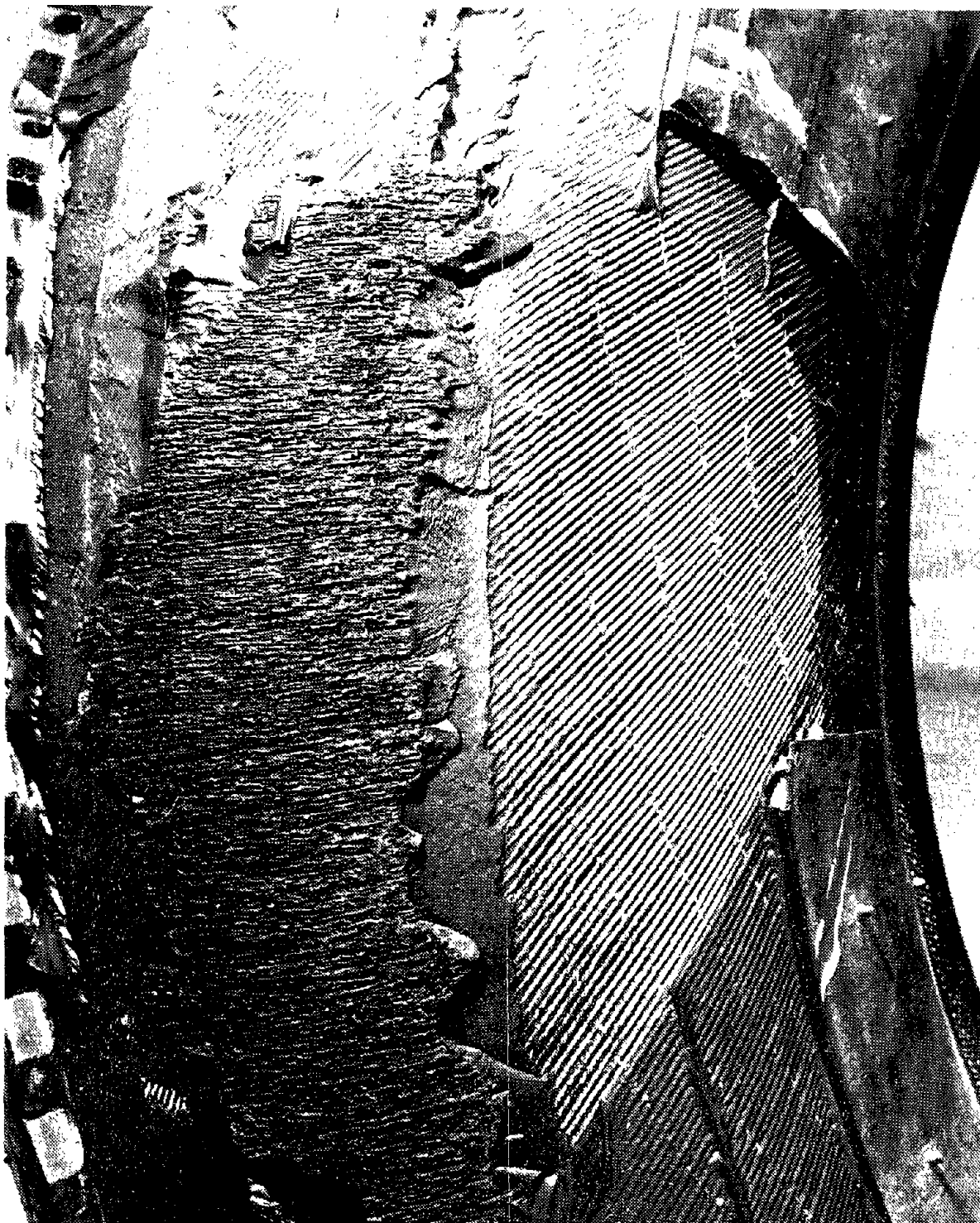
Figure 1. Sidewall Separation and Area of Poor Rubber Adhesion T5X 1161
