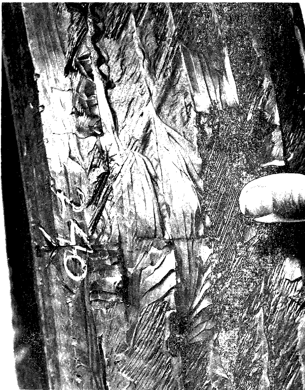
Figure 4. Severe Belt Breakage and Separation in Failure Area T5X 1204
