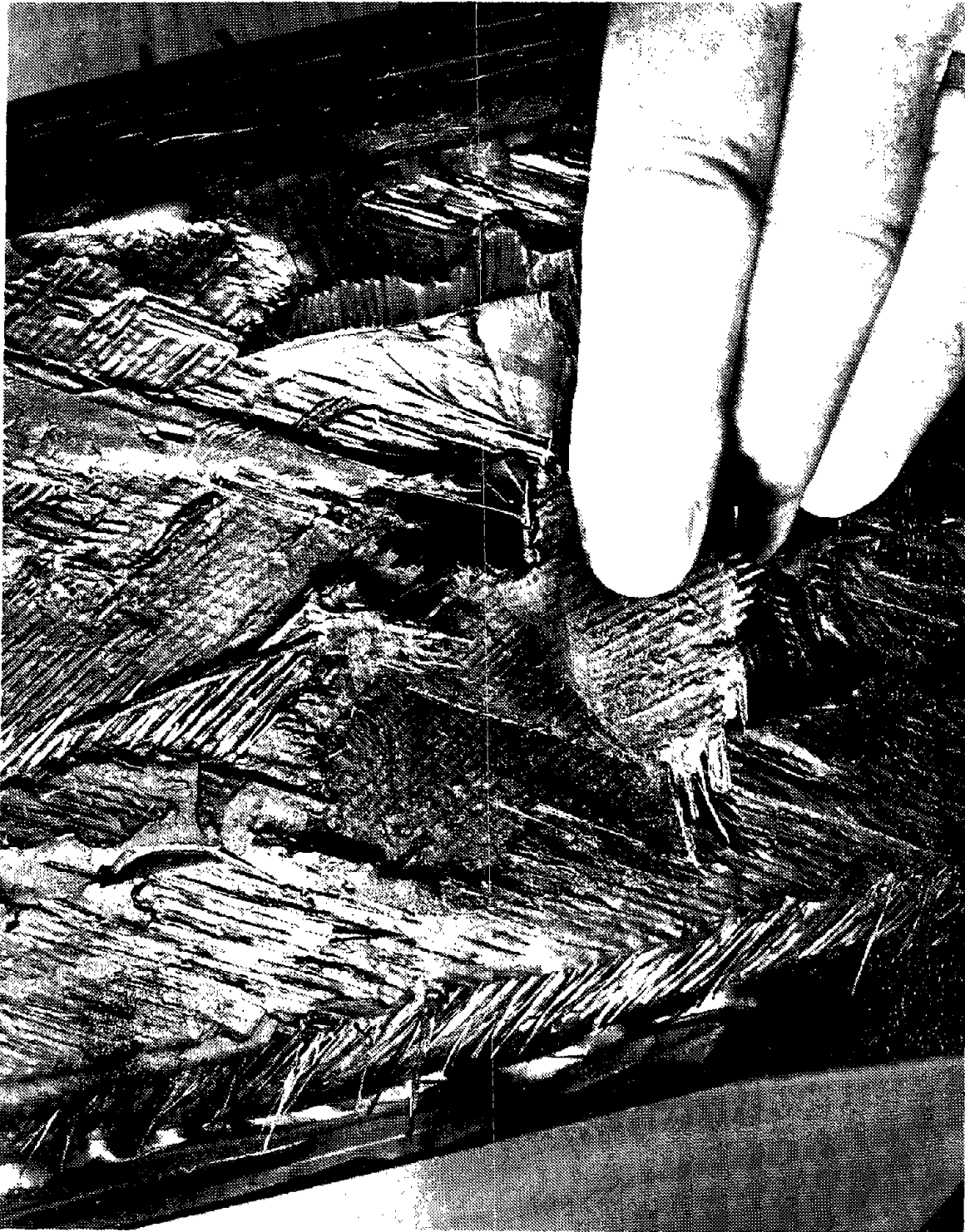
Figure 2. Severe Belt Breakage and Failure Area T5X 1183
