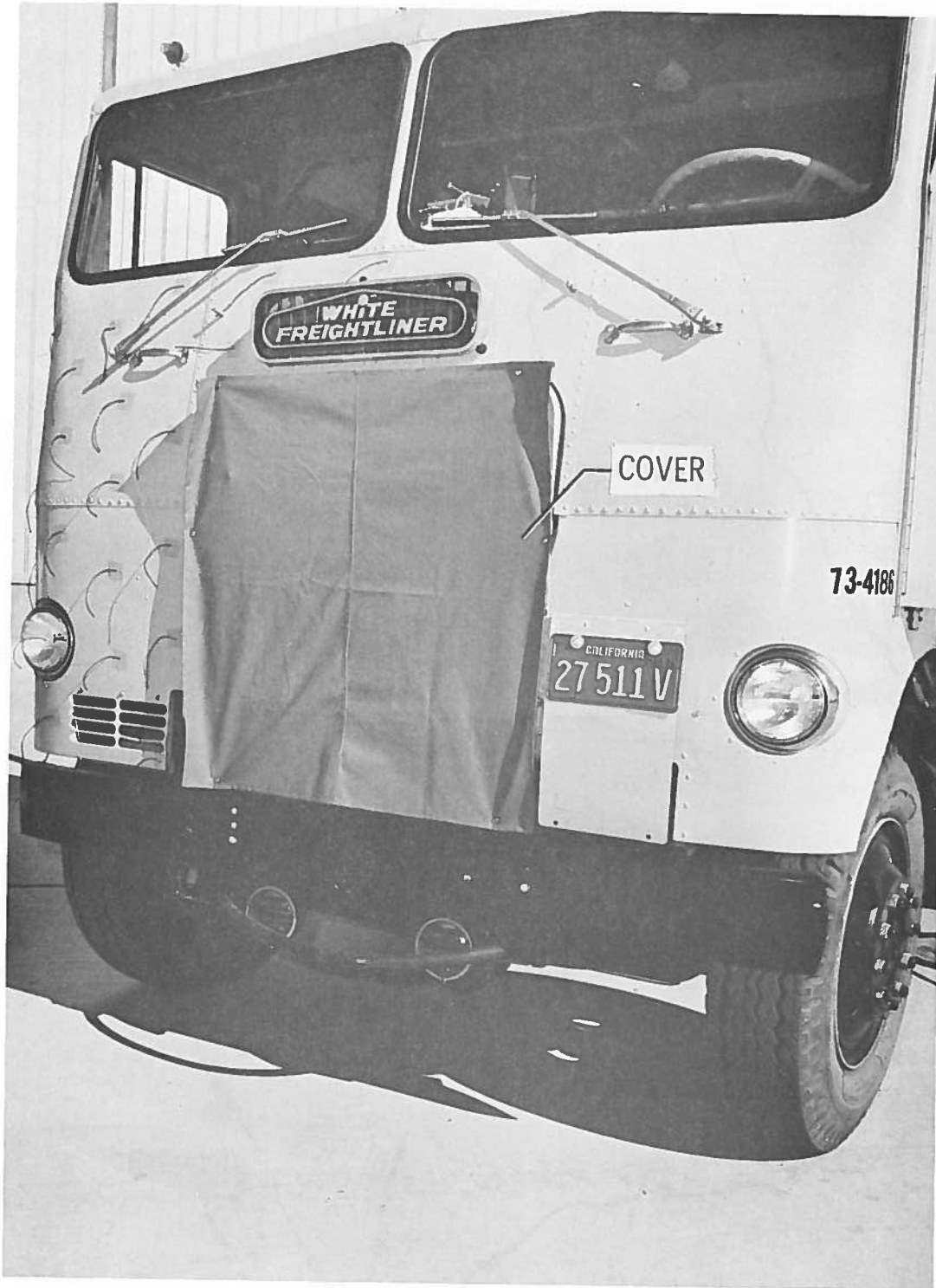
FIGURE 2. COVER OVER RADIATOR OPENING
