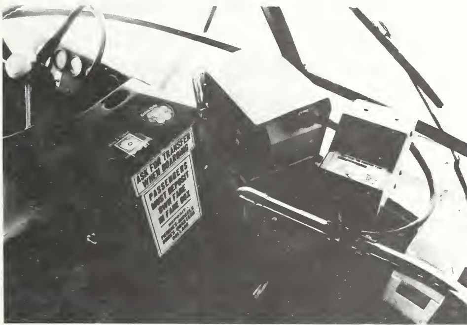
FIGURE 3.5 TOP VIEW OF AN AFIR SHOWING LOCATION RELATIVE TO EXISTING FAREBOX AND DRIVERS SEAT
