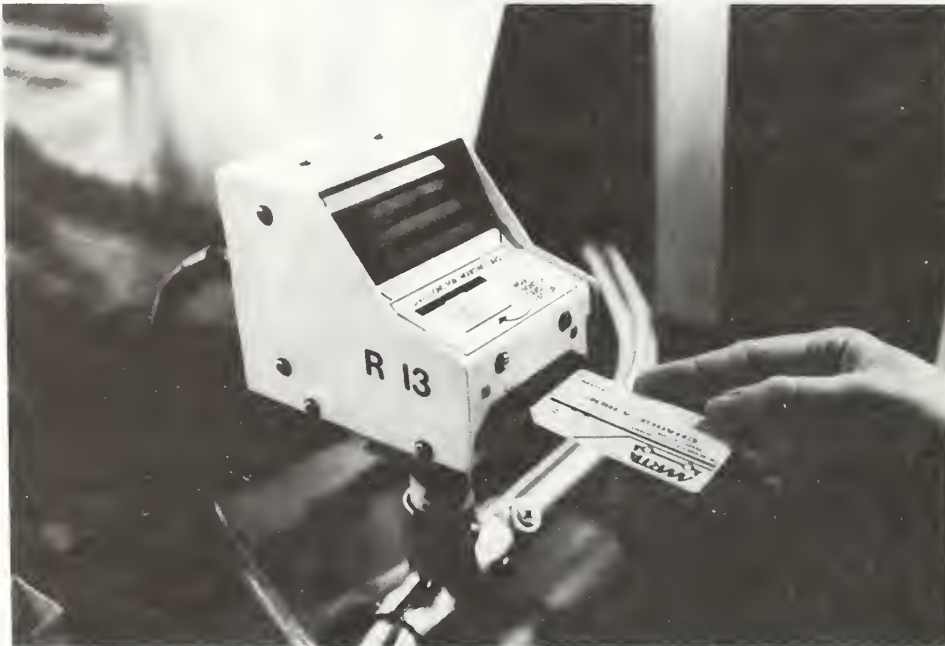
FIGURE 3.4 VIEW OF AN AFIR CARD READING MECHANISM IN USE
