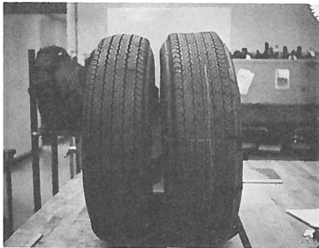
Figure 3-6. Tires of Different Size Retreaded and Cured in the Same Mold
