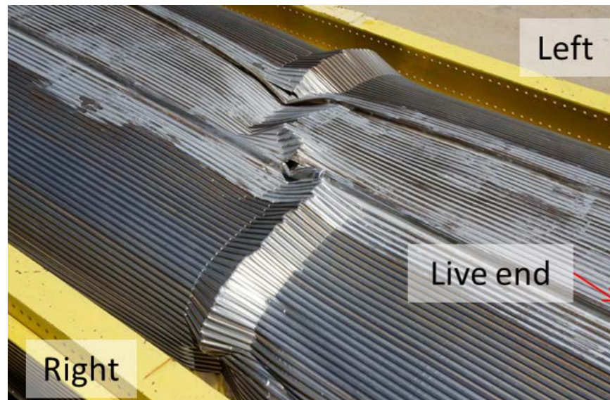
Figure 53. Buckled Roof, Car 248
