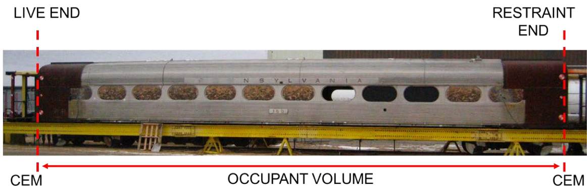
Figure 7. Car 244 in Test Frame, 800-kip Verification Test
