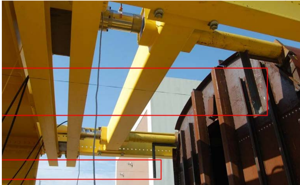
Figure 36. Typical Longitudinal String Potentiometer Setup, Car 244
