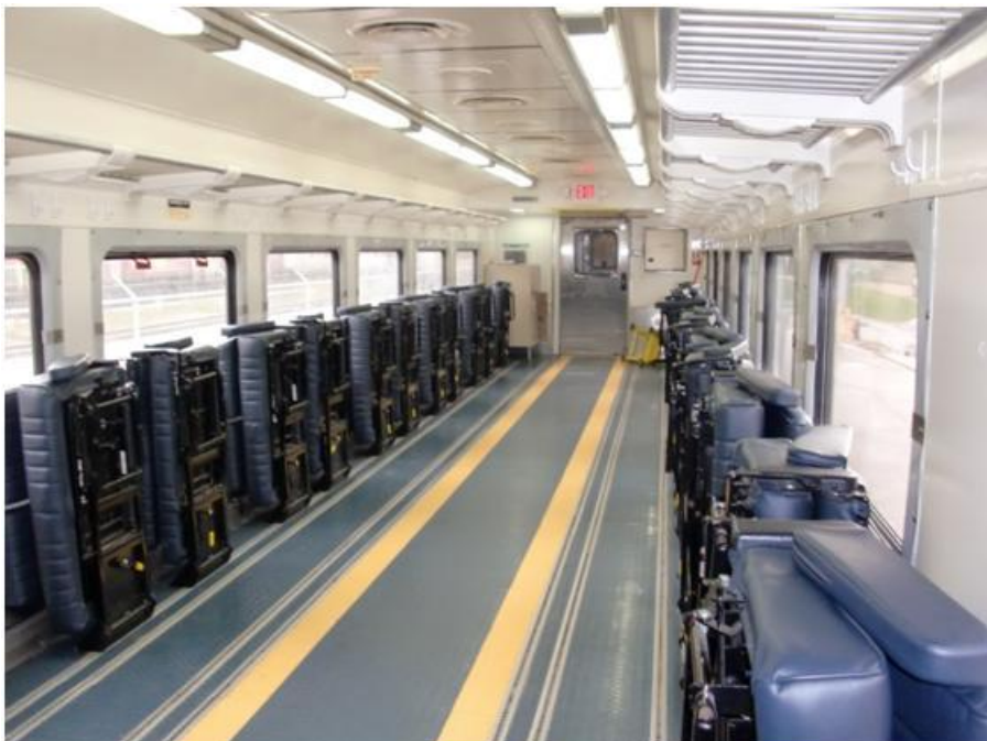
Figure 36 Interior of accessible car 105 Source: Volpe Center
